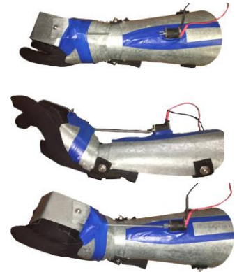
Figure 30: ARCTiC LawE Vrs. 2 (Top) Top down view - unactuated (Middle) Side view - actuated (Bottom) Top down view - actuated
